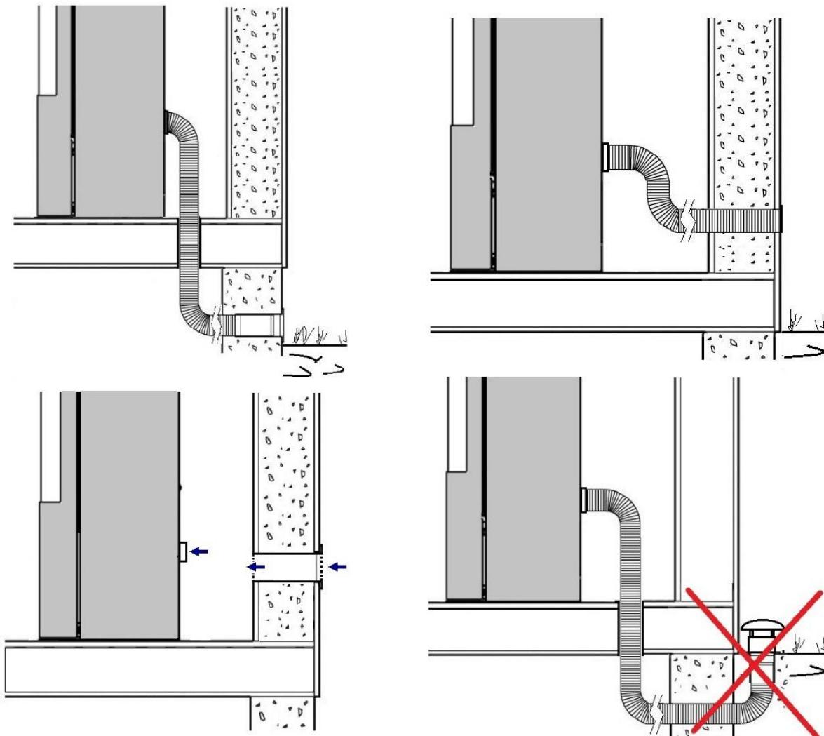
If there are any problems with the functioning of the chimney, these must be solved before installing the stove.
