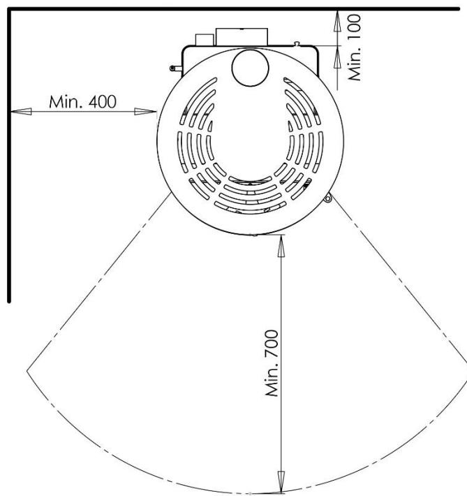
To secure access to inspection openings and enough air for the combustion, there needs to be a distance of at least 10 cm to the wall behind and 40 cm to the side. You must be prepared to dismount the flue pipe and turn the stove during the yearly inspection and by maintenance.
